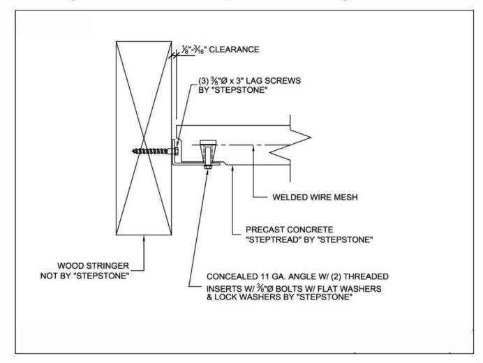
PRECAST CONCRETE TREADS AND LANDINGS SHOWN ON PLANS SHALL BE FROM THE "STEPTREAD" SYSTEM BY STEPSTONE, INC. OF GARDENA, CA, FOR WOOD CONSTRUCTION. THE MANUFACTURER IS TO SUPPLIY ALL PRECAST CONCRETE PARTS WITH EACH "STEPTREAD" INCLUDING ALL GALVANIZED HARDWARE SHOWN IN THIS SERIES, TO ATTACH SAME.
