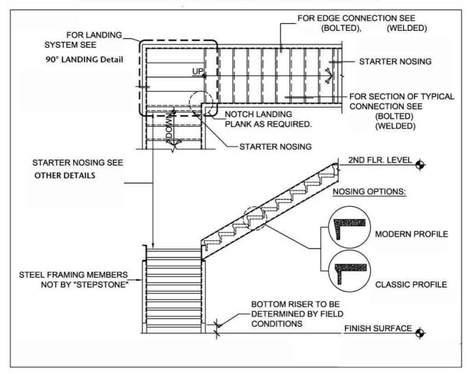
PRECAST CONCRETE TREADS, LANDINGS, AND BALCONIES SHOWN ON PLANS SHALL BE FROM THE "STEPTREAD" SYSTEM BY "STEPSTONE, INC." OF GARDENA, CA. FOR STEEL OR WOOD CONSTRUCTION. THE MANUFACTURER IS TO SUPPLY ALL PRECAST CONCRETE PARTS WITH EACH "STEPTREAD" AND FEATURING EITHER CAST IN THREADED INSERTS FOR BOLTING OR AN EMBEDDED BOTTOM WELD PLATE FOR WELDING.
